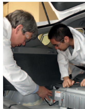
Chris Phyland and Rob Dark work on converting a Toyota Prius into a plug-in hybrid electric vehicle. CSIRO
